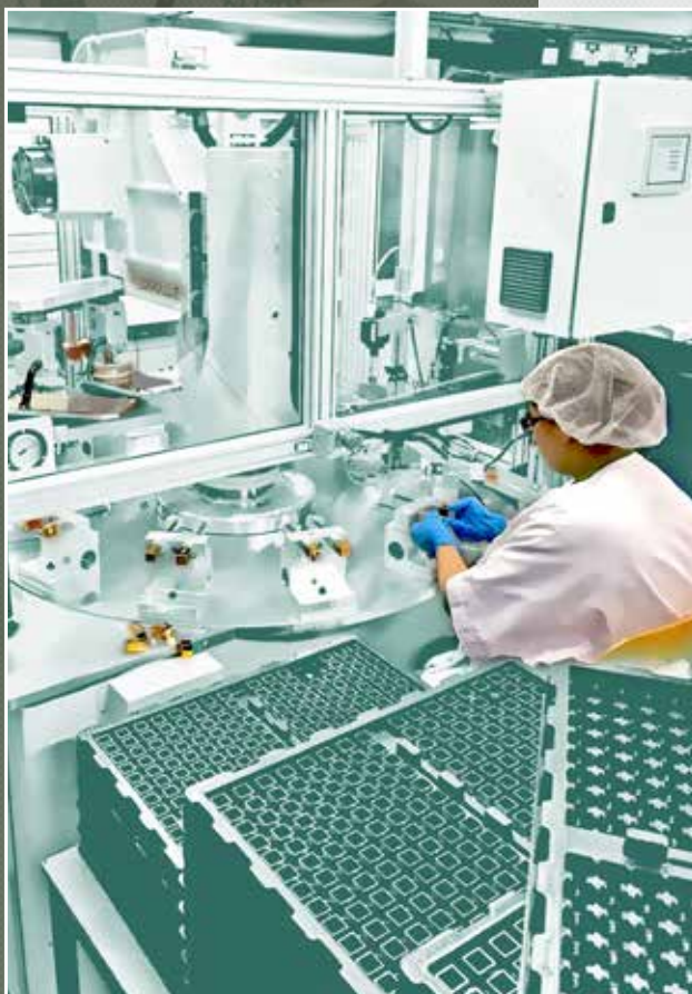
Logica Platform mod. S N. 1 print head Logica Micro II with protruding rotary table, to facilitate the manual loading and unloading of the pieces.
